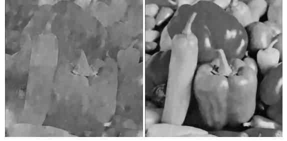
Fig. 5. Left: reconstructions from sampling uniformly at random (plus the zero frequency sample) at 10% with a relative error of 0.33. Right: reconstruction from sampling in the semi-uniform random manner described in Theorem II.4 at 10% with a relative error of 0.07.
